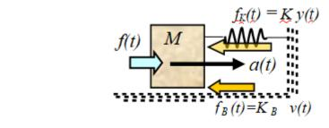
$$M\frac{d^{2}y(t)}{dt^{2}} = f(t) - f_{B}(t) - f_{K}(t) = f(t) - B.\frac{dy(t)}{dt}(t) - Ky(t)$$
