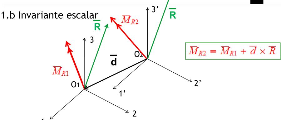
$$M_{R2}^* = \overline{n}_R \cdot \overline{M}_{R2} = \overline{n}_R \cdot (\overline{M}_{R1} + \overline{d} \times \overline{R}) = \overline{n}_R \cdot \overline{M}_{R1} + \overline{n}_R \cdot (\overline{d} \times \overline{R})$$
