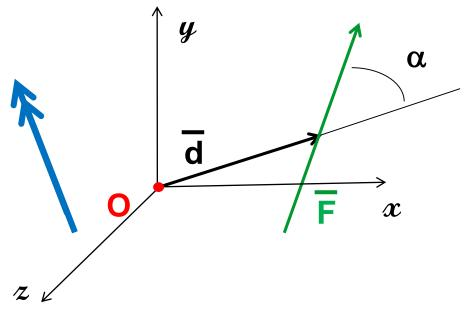
$$\overline{M}_F^O = \overline{d} \times \overline{F} = \begin{bmatrix} i & j & k \\ dx & d_y & d_z \\ F_x & F_y & F_z \end{bmatrix} = (F_z d_y - F_y d_z) \hat{i} + (F_x d_z - F_z d_x) \hat{j} + (F_y d_x - F_x d_y) \hat{k}$$
