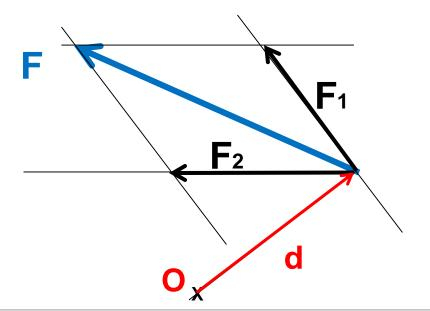
$$\overline{M}_{O,F} = \overline{d} \times \overline{F}_{1} + \overline{d} \times \overline{F}_{2}$$
